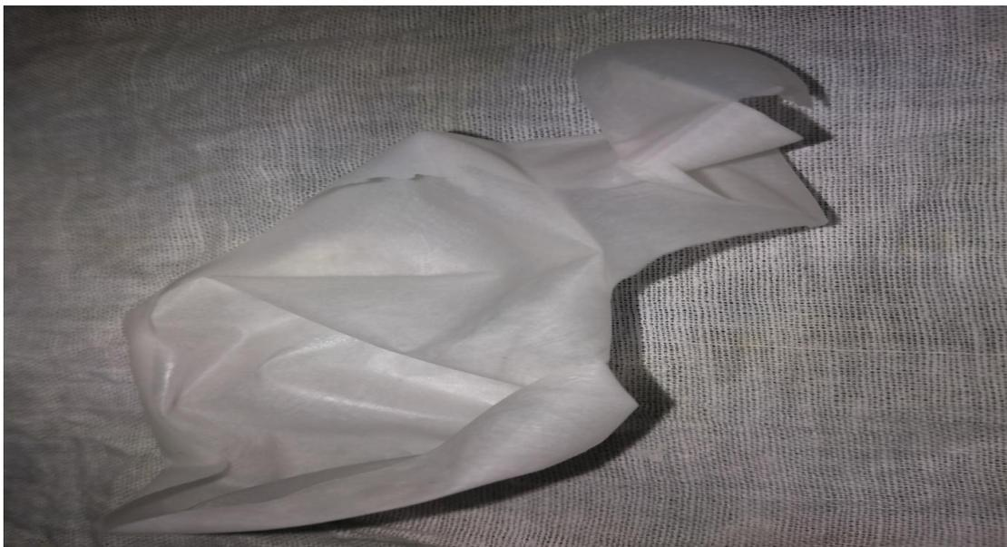
Fig. 3. Prepared semipermeable membrane from egg
